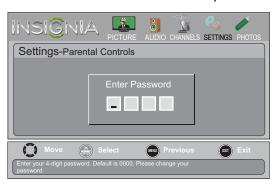
**4** Press the number buttons to enter the four-digit password. The default password is **0000**. You should change the password to a number you can remember. The *Settings-Parental Controls* menu opens.
